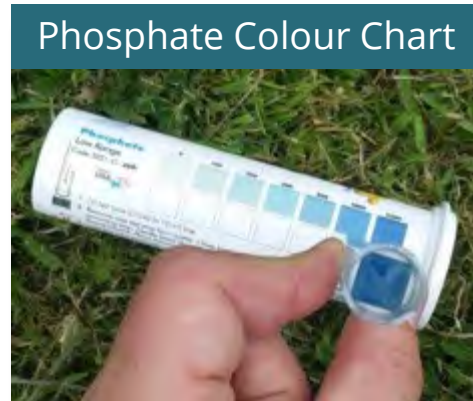
Phosphate Strip being inverted in sample
